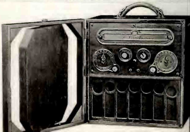
RCA portable of 1926 weighed 60 pounds. Loop in front cover. Six tubes. Price, $225 with home unit for larger batteries.
