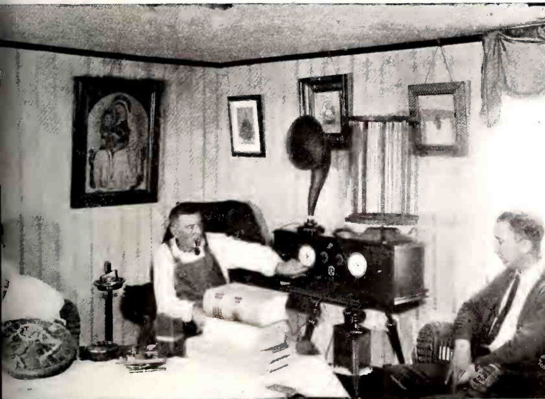
A GE receiver of 1923 being used by a farm family. Note rotative loop antenna and goose neck speaker which could be plugged into different audio stages.
