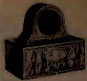
Early AC-operated receiver was this Stewart-Warner model 802. Seven tubes. Power-line aerial. $110.50.
