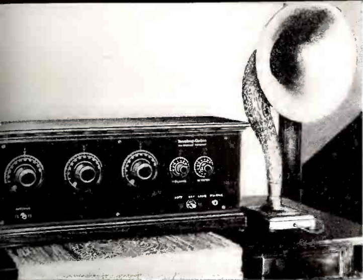
Stromberg-Carlson set with Neutrodyne circuit and famous "goose magnetic speaker. RF and detector stages were individually tuned.
