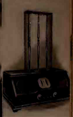
Six-tube superhet of 1925, a Radiola 25. Single control tuning. Price $165 with tubes.
